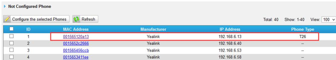
**Step5.** Assign extensions to the phone, and you can also configure the Memory keys and Line keys.
